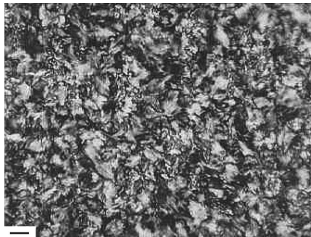
Fig. 7. OM of the LPE component. The sample experienced a cooling rate of 1^{\circ}\text{C min}^{-1} prior to examination in OM. The scale bar in the picture is 10\ \mu\text{m} .
